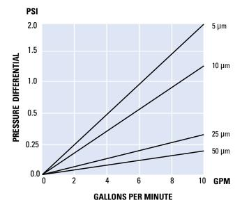
Flow rates exceeding 7-8 GPM per 10" length are not recommended for 50 microns or below for maximum service life. This chart represents the typical flow rate per 10" cartridge length. The test fluid is water at ambient temperature. Extrapolations for multiple lengths tend to be linear, but as flows increase the differential pressure across the housing becomes more apparent.
