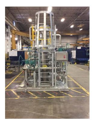
For heated gaseous fuel applications Hilco manufacturers hi temperature filter/separator versions for continuous operation up to 500 F (260 C).
