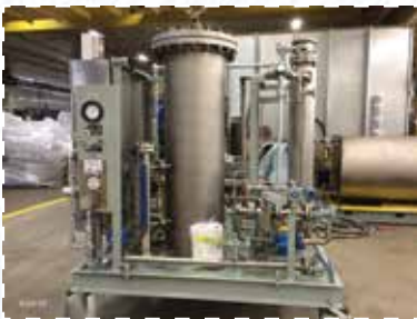
Ex: Stainless and Carbon Steel heated system with Pre-filter. Explosion-Proof with purged electrical enclosure and transmitters. 2014
